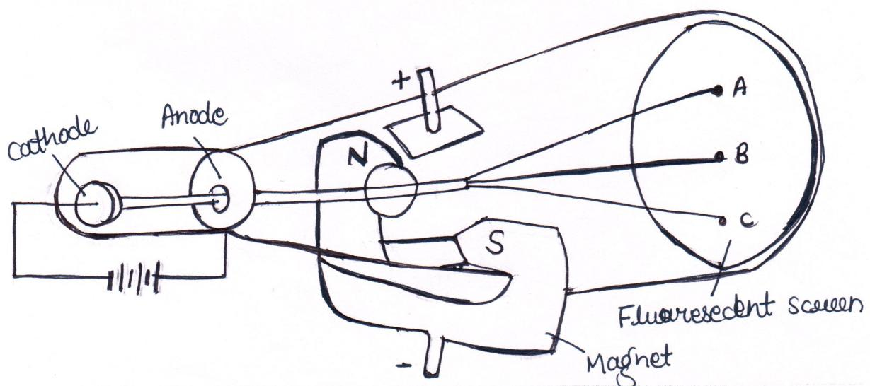
The amount of deviation of the particle from their path in the presence of electrical or magnetic field depends upon:
